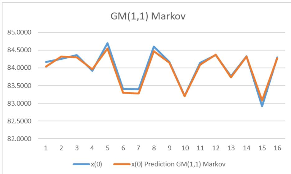
**Figure 8. Actual and Predicted Values According To GM (1,1) Markov Model For The Sterilizer Temperature**
