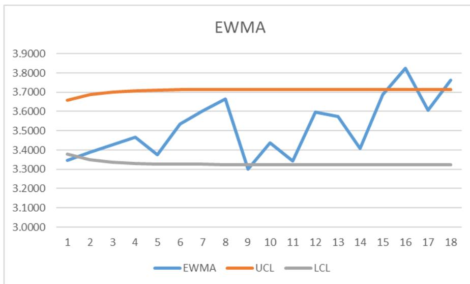
**Figure 10. EWMA Quality Control Chart for the Grid-Pan Temperature**
