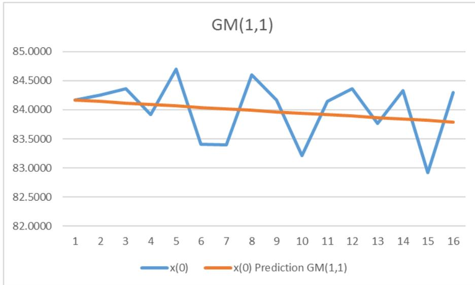
**Figure 7. Actual and Predicted Values According To GM(1,1) Model For The Sterilizer Temperature**
